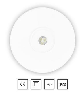
EXISAFE-3T is powerful surface-mounted LED emergency luminaire for spaces where ceiling height exceeds 10 m. EXISAFE-3T/120, on the other hand, is designed for ceiling heights of under 10 m. Light fitting delivers a wide, rotationally symmetrical light pattern. IP55 rated luminaire is also well suited for emergency lighting in humid locations. It has an ABS plastic body. The standard colour for the plastic parts is white (RAL9016).
